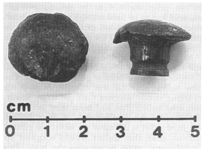
FIG. 3. Two Vetterli rifle bullets recovered from 10 per cent ordnance gelatin. Lengths of these bullets were 13.6 and 15.0 millimeters; the Vetterli rifle bullets recovered by Kocher from a box filled with water were 14 millimeters long.
